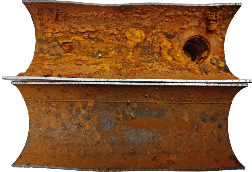
FIGURE 2; 1 Pipe Sample Sectioned: 2.5" Black Iron Schedule 10 Pipe
